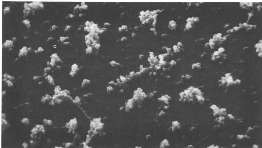
Figure 11a. SEM photomicrograph of copper–2% zinc alloy exposed for 4 h in 4 g/L of human fibrinogen phosphated saline solution at 25 o , pH 7.4, by immersion only.
