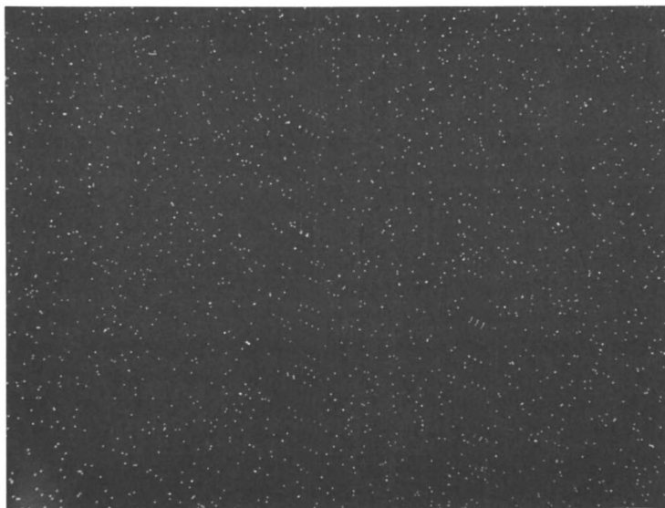
Figure 1b. Phosphorus x-ray dispersion map of PNF as cast from acetone at 0 h irradiation.
