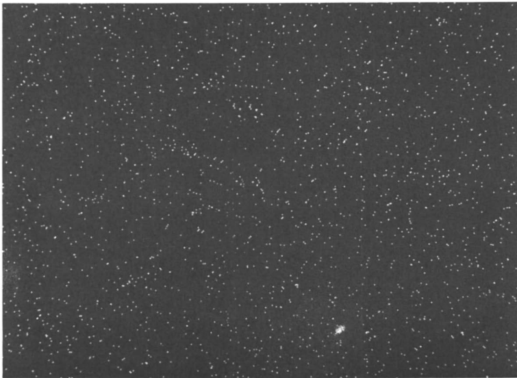
Figure 3b. Phosphorus x-ray dispersion map of PNF as cast from acetone at 24 h irradiation.
