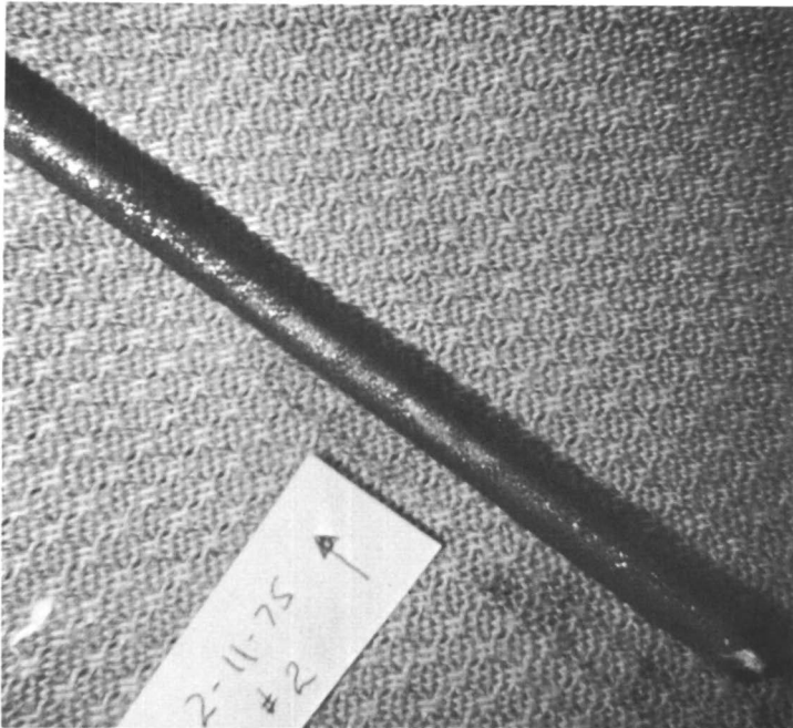
Figure 3. Typical pattern of uniform thrombus formation over entire surface of biomaterial coated rod (4).
