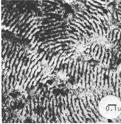
Figure 2. TEM of the phase-separated, (dioxane-cast) osmium vapor-stained triblock copolymer. The stained (dark) regions are the ATBN midblock segments and the unstained regions are the BLG segments of the block copolymer.
