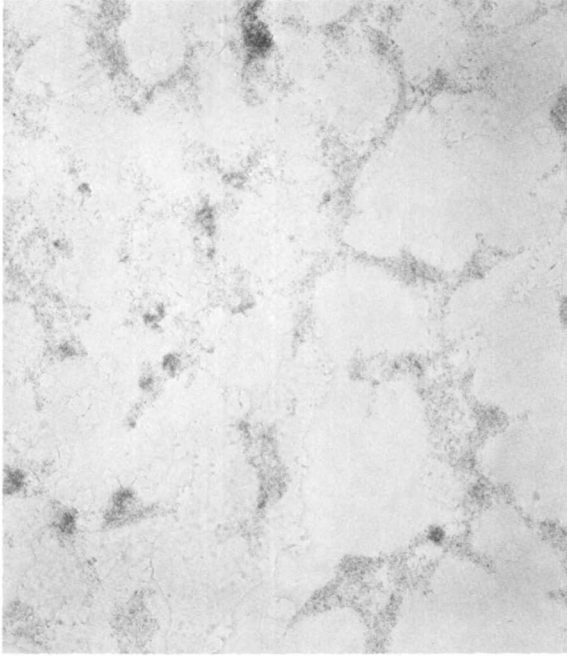
Figure 3c. The \gamma -globulin adsorbed on the sintered Teflon sample of Figure 2a (dry air technique). Rabbit anti-BSA (IgG), 250 mg/dL, ferritin label, TEM, higher magnification. Key: bar equals 1 \mu\text{m} .
